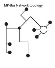
There are no restrictions for the network topology (star, ring, tree or mixed forms are permitted). Supply and communication in one and the same 3-wire cable • no shielding or twisting
